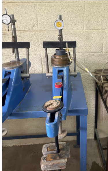
Figure 6. Collapse test setup
