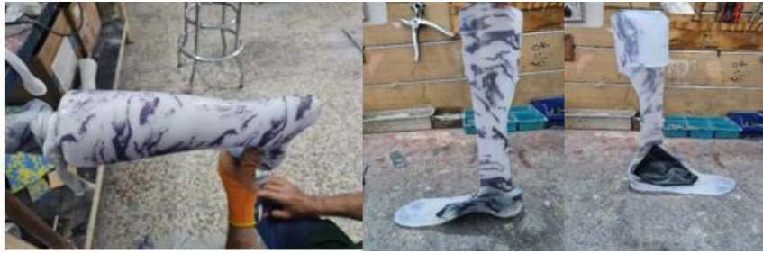
Figure 10. Designing the orthosis base
