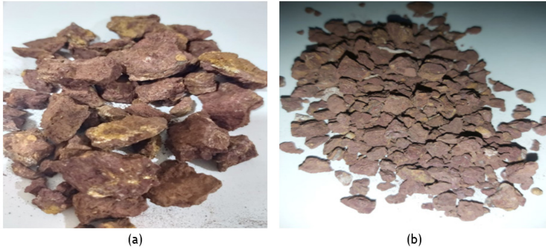
Figure 2. Particle size of the sample : (a) before crushing. (b) after crushing.
