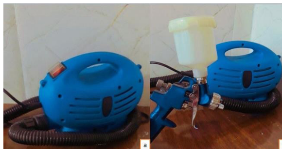
Figure 3. (a) air compressor for spraying with an airbrush, (b) the system of the spray airbrush gun
