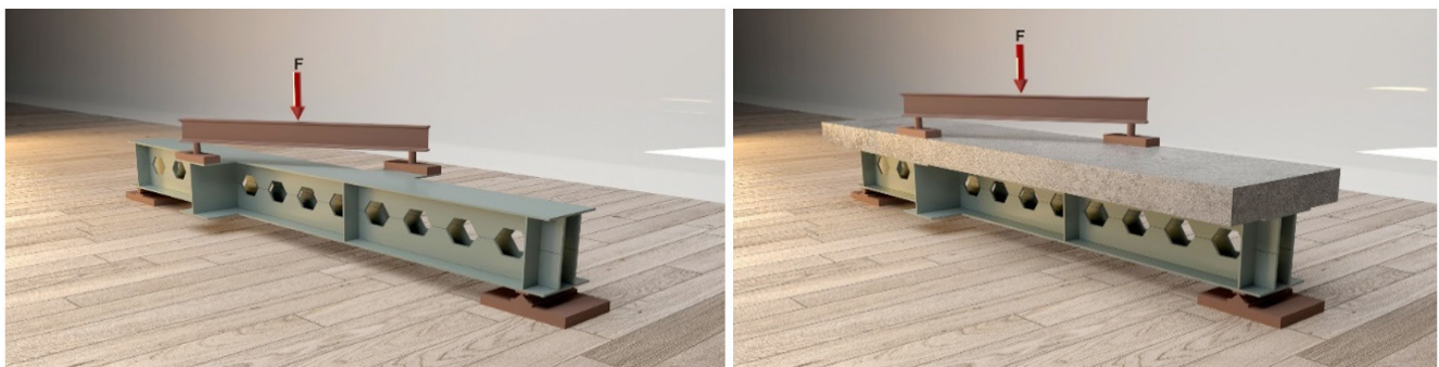
Figure 2. Specimens under Combined Load
