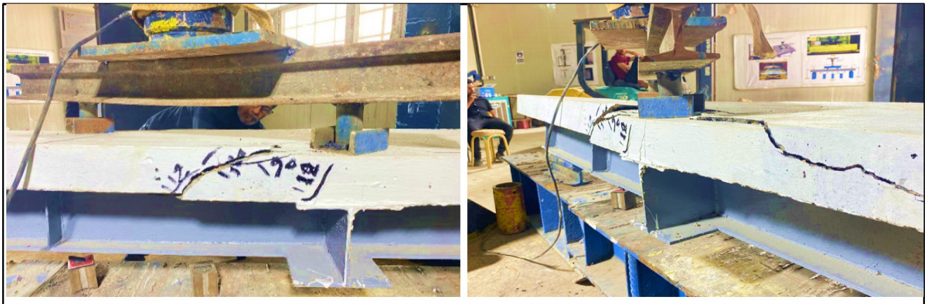
Figure 8. Failure of composite specimens under combined (FT)
