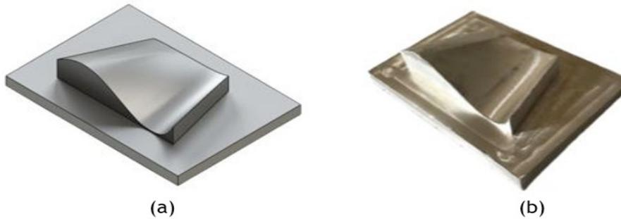
Figure 4. (a) A SOLIDWORKS die design and (b) final milling die
