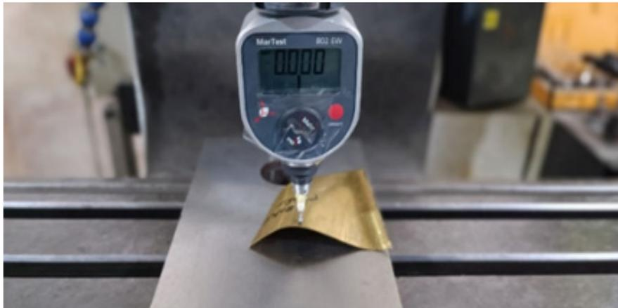
Figure 14. Accuracy test via NC milling machine
