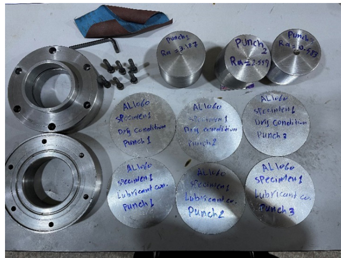
Figure 4. The Nakajima die with three hemispherical punches and six circular Aluminium AA1060 blanks
