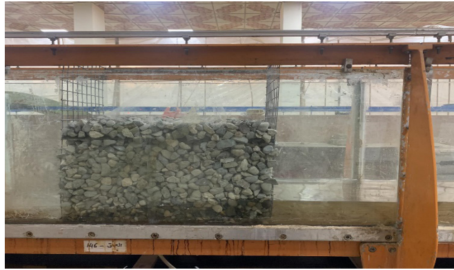
Figure 3. Hydraulic gradient through Self-Spillway dam at low discharge value
