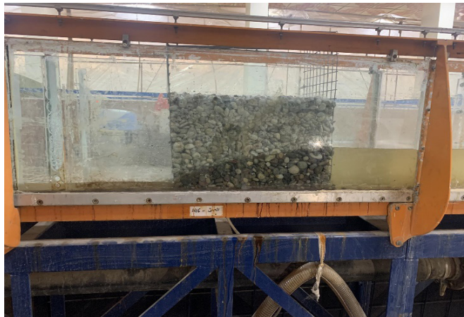
Figure 4. Hydraulic gradient through Self-Spillway dam at an increment of discharge value
