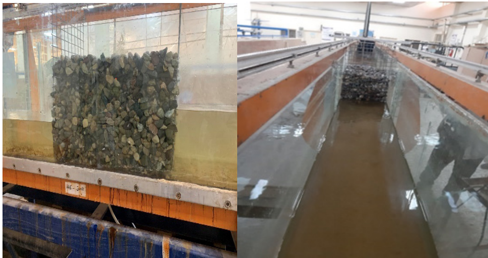
Figure 2. Self-Spillway dam model
